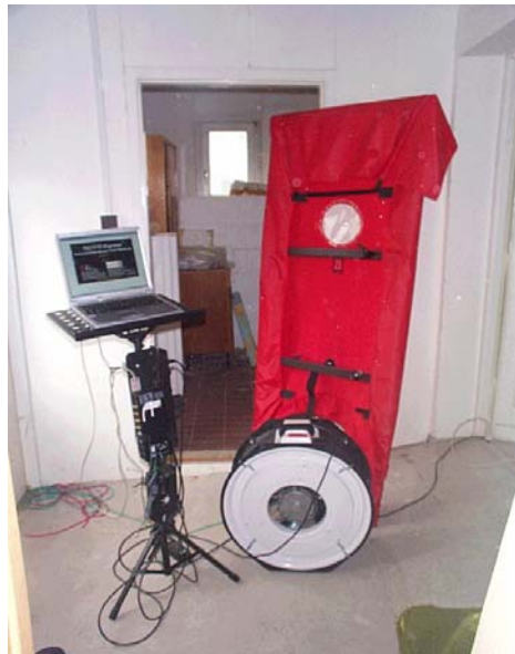
Figure .: Air-tightness test of a timber house
