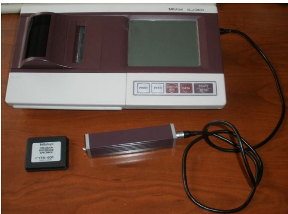
Fig. 6: Surftest SJ-301 surface roughness-meter
