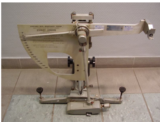
Fig. 3: Skid Resistance Tester
